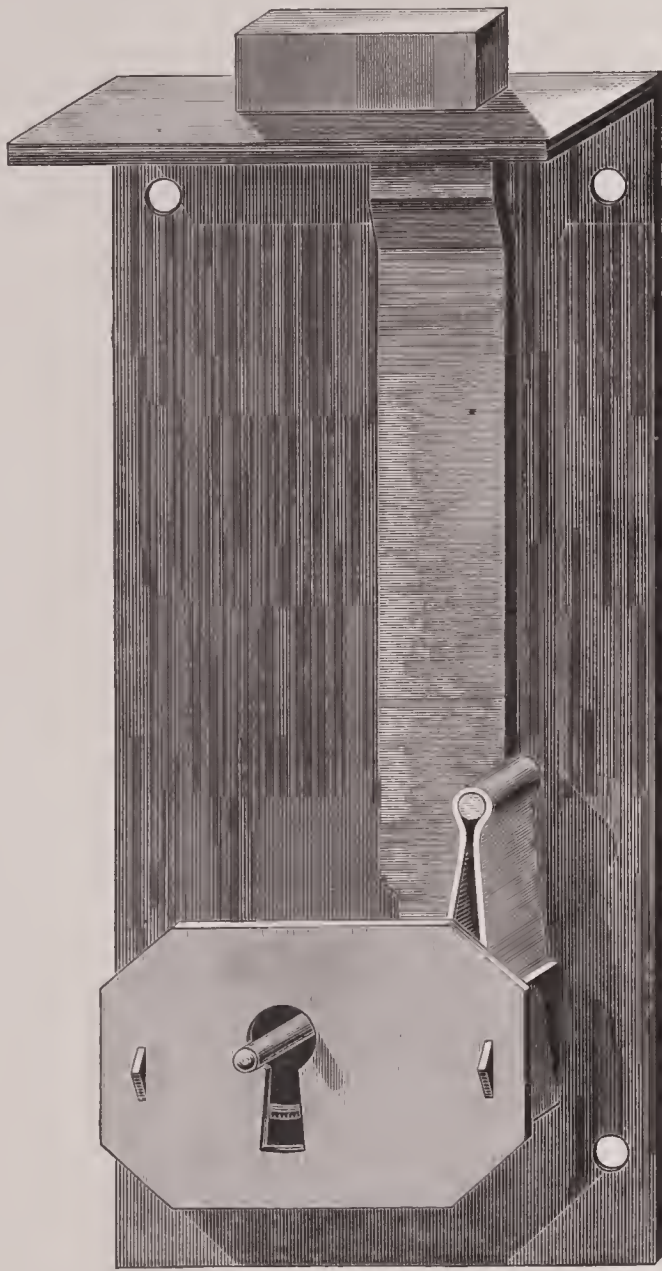
No. 42 I, A. 2½ inch, $3.60. Iron. Square Brass Selvedge, Broad Heavy Bolt, Tumbler, 1 Ward. 4½ inches from Selvedge to middle of Key-hole.
